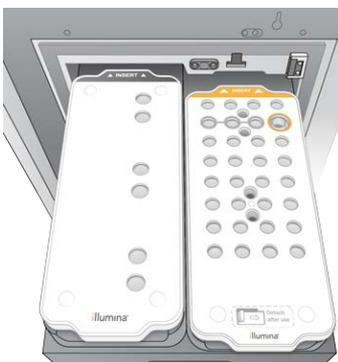
5. Slide the drawer into the chiller, and then close the reagent chiller door.
