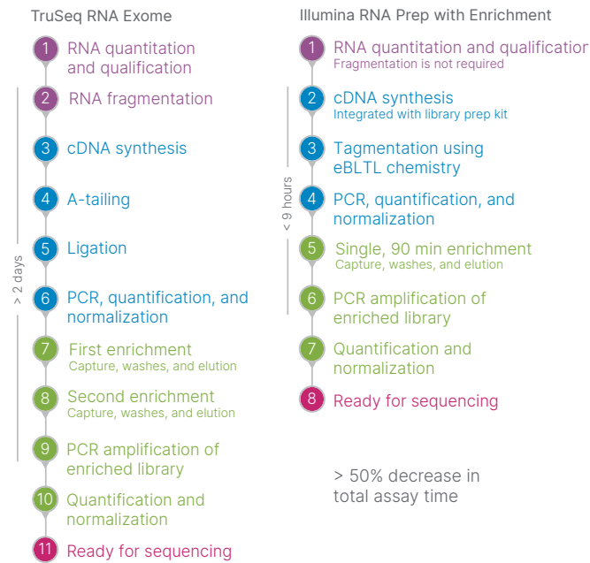
Figure 1: TruSeq RNA Exome and Illumina RNA Prep with Enrichment workflows—On-Bead Tagmentation and a single, 90 minute hybridization step combine to deliver a faster workflow with fewer steps when Illumina RNA Prep with Enrichment in comparison with TruSeq RNA Exome
